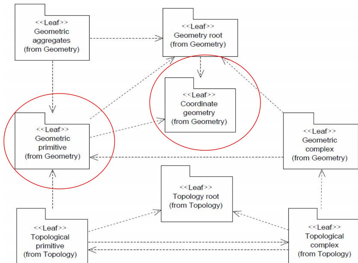
Figure 4: ISO 19107 Geometry packages (Red circles for the subset of the ISO 19137 core profile)
