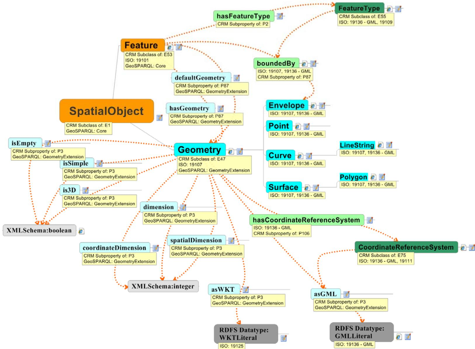
Figure 3: GeoSPARQL Core Component and Geometry Extension with CIDOC CRM and ISO relations
