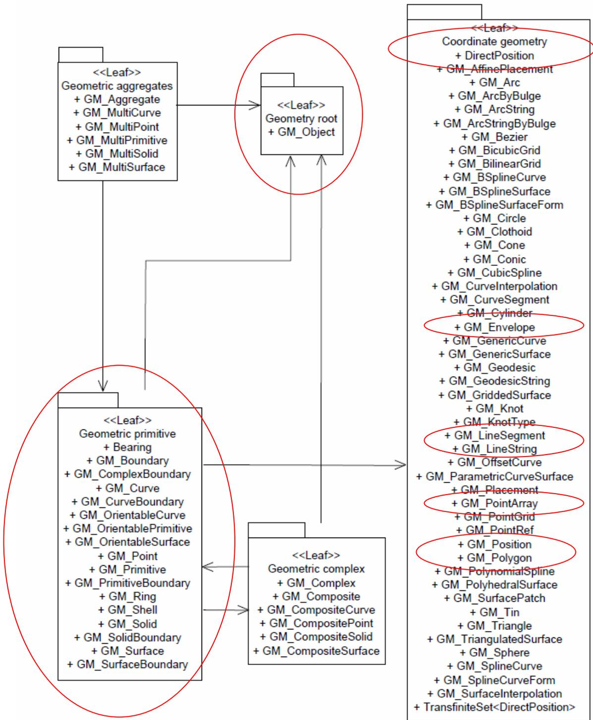
Figure 5: Geometry package: Class content and internal dependencies (Red circles for the subset of the ISO 19137 core profile)
