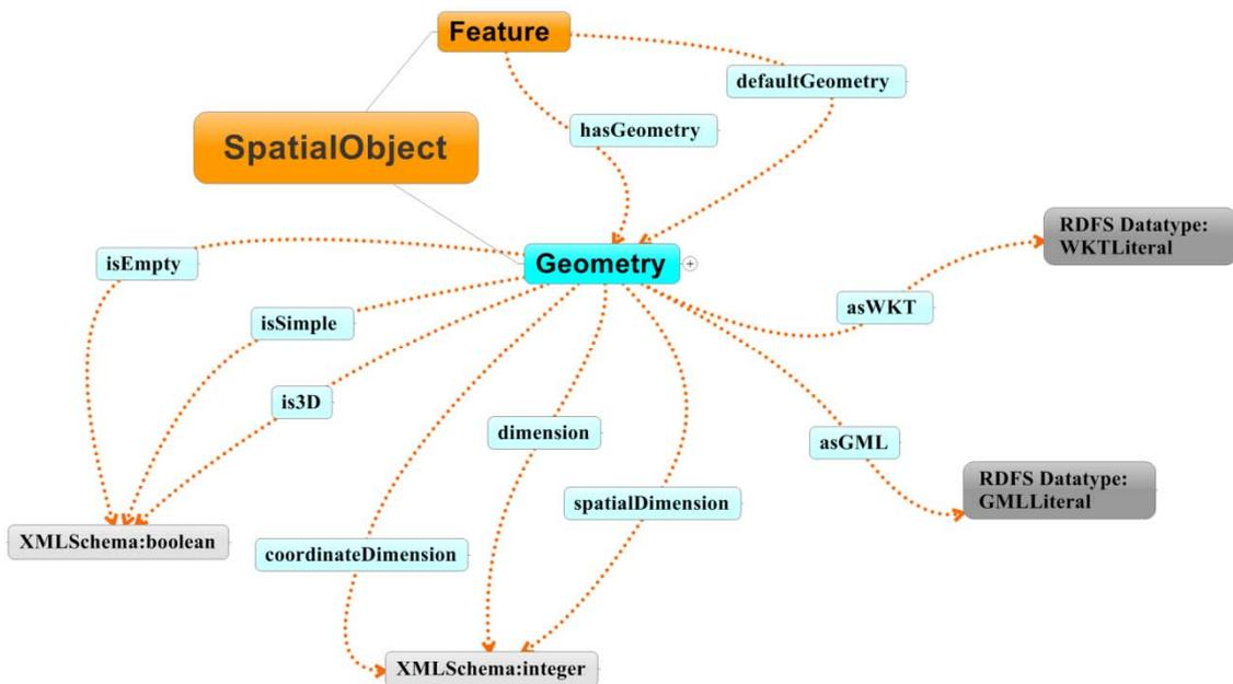
Figure 2: Core component classes (SpatialObject, Feature) and Geometry Class with properties
